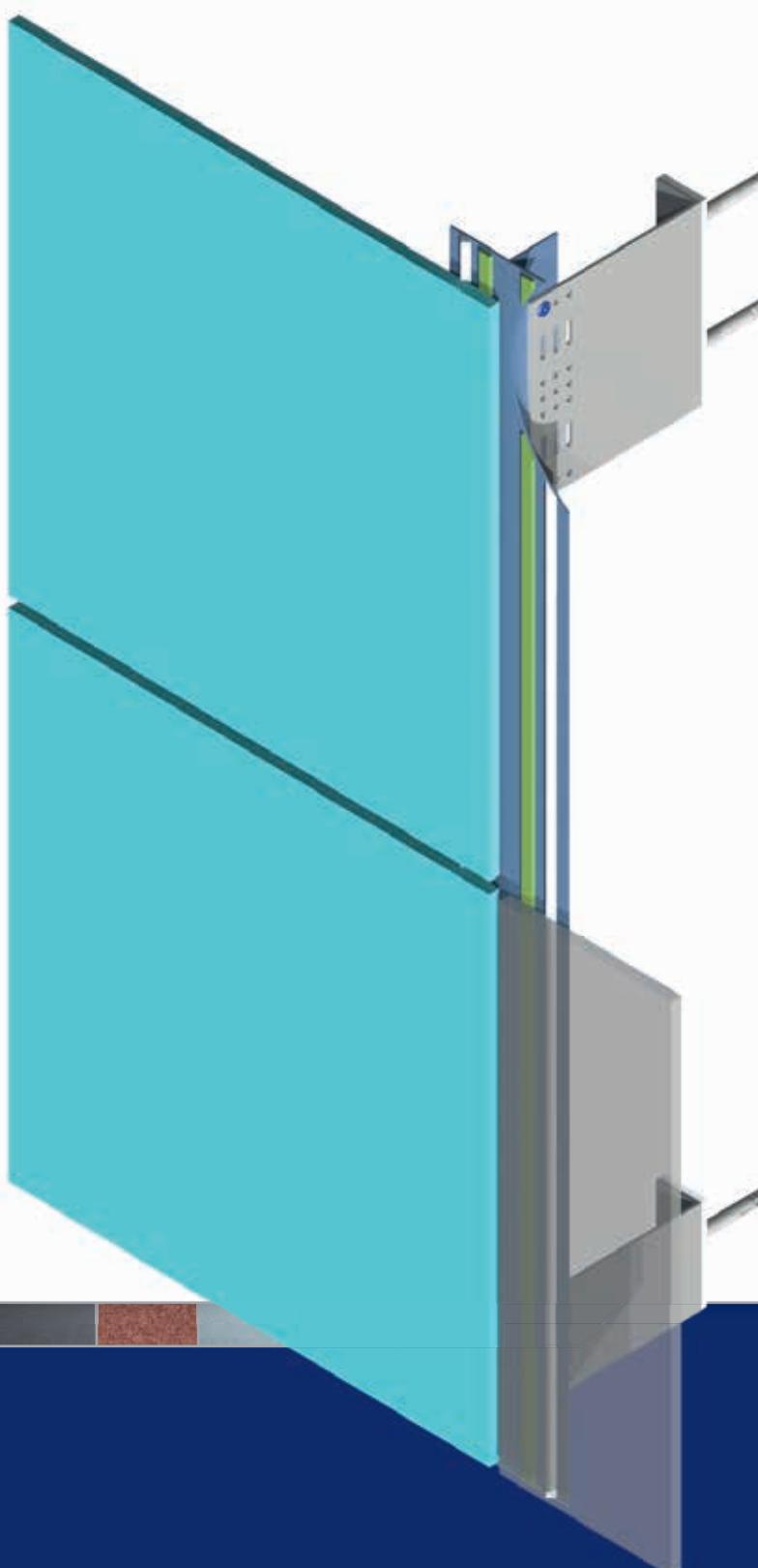
System: **ALWI**      holding tracks for glued-on wall panels
